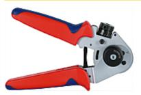
Crimping tool for crimping turned contacts. Four-manderel crimping. Fine adjustment of pressure depending on the conductor's diameter by means of adjusting wheel. Can be used to 0,08 - 2,5 mm². High crimping quality due to to integral lock.
