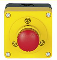
PITestop E-STOP/contact block incl. surface mount housing, set consisting of E-STOP pushbutton with E-STOP symbol and with logo and contact block with monitoring, 2 N/C, terminals of screw type.
