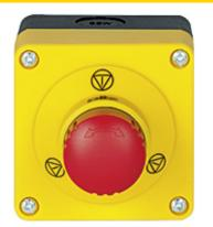
PITestop E-STOP/contact block incl. surface mount housing, set consisting of E-STOP pushbutton with E-STOP symbol and with logo and contact block with monitoring. 2 N/C, 1 signal contact (1 N/O, 2 N/C), terminals of screw type.
