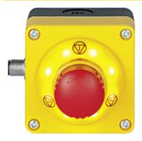
PITestop E-STOP/contact block incl. surface mount housing, set consisting of illuminated E-STOP pushbutton with E-STOP symbol and with E-STOP symbol and with logo and contact block, 2 N/C, with M12 connection 5-pin.
