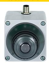
PITestop set consists of active/non-active E-STOP push button with flashing feature without Pilz label, without emergency stop symbol, with LED safe module and with contact block in basic surface mounted housing with M12/5pin connector compatible with PDP67 8DI ION; complies to EN 60947-5-1 and EN 60947-5-5; 2 n/c; spring terminals.
