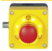
PITestop E-STOP/contact block incl. surface mount housing, set consisting of illuminated E-STOP pushbutton with E-STOP symbol and with E-STOP symbol and with logo and contact block, 2 N/C, with M12 connection 5-pin compatible with AIDA.
