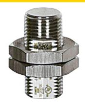
Safety switch for movable guard's position monitoring in accordance to EN 60947-5-3; for applications up to SIL3/PL e/Cat4; M12 design; IP69; Content= 1 actuator M12; Sao=8mm; stainless steel housing; ATEX Approval
