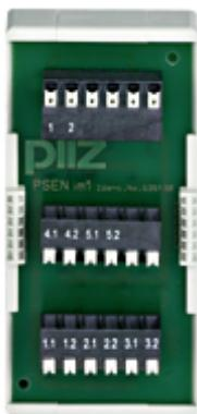
Interface PSEN im1 for connection and evaluation of several Pressure sensitive mats to the PNOZmulti system; 96 x 48 x 43.5 mm (H x W x D); connection type spring-loaded terminals.
