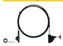
push-pull-cable release for safety gate system PSENmlock; cable length 0.75m; Content = push-pull-cable with operating element and mounting accessories Ensure that these versions are installed as straight as possible. On escape releases with order no. 570466 and 570467, bending the push / pull cable may reduce ist functionality and lifetime.
