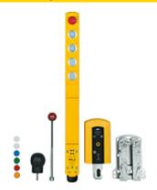
Safety gate system includes safe interlocking device with guard locking. According to DIN EN60947-5-3. For applications up to SIL CL3 or Ple. Device type: 1. blind cover 2. blind cover 3. illuminated push button 4. illuminated push button 5. E-Stop Scope of delivery: Sensor unit with push buttons including color covers and escape release pin as well as actuator (bolt) for doors with hinges left or right.
