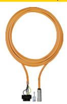
Cable for PMCprotego and motor with connector design assembled on both sides with connector <> round connector 8-pin No. of wires and cross section  $(4 \times 4.0 + (2 \times 1,5))$  Trailing, length: 20 m.
